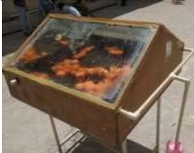
Figure 6: Experimental Set up of solar still
