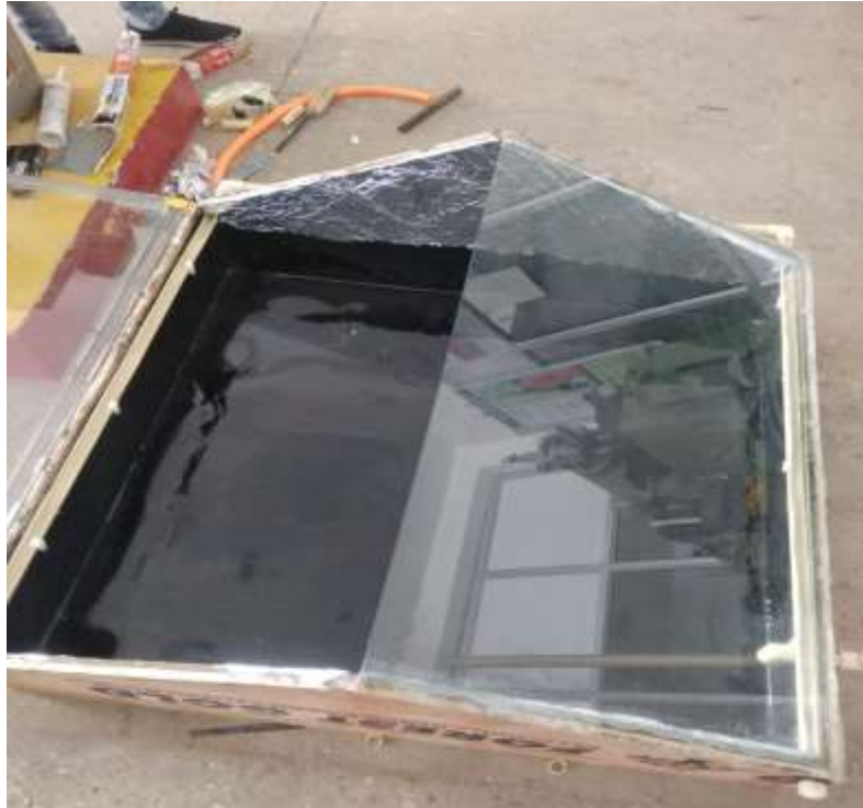
Figure 1: Fabrication of Double slope solar still
